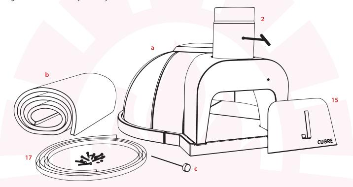
The **Cuore 1000+ Wood-Fired Oven Kit** consists of the refractory numbered oven parts (a), including the chimney tube with incorporated flue damper (2), the three steel belts and related hardware (7 bolts measuring ½" x 2.1/2", 7 washers, 3 nuts) (17), the oven door (15), a rock wool thermal blanket (b), a thermometer (c) and this Assembly Manual, which is available online on <a href="https://www.cuoreovens.com">www.cuoreovens.com</a> so you can always have the most up-to-date revision.
